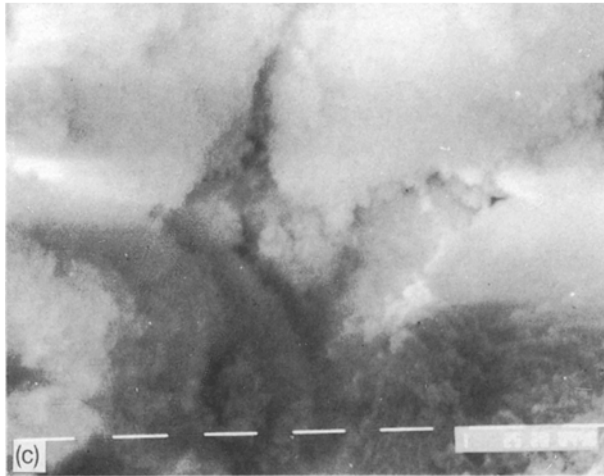
Figure 4 Scanning electron micrographs of the Mg, Al-hydrotalcite material after heat treatment at 725 °C (a) \times 1000 (b) \times 5000 and (c) \times 10000 .
